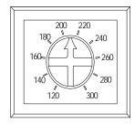
**Note:** To protect the motor, set the arrow number as the same as the motor nominated power. Whenever overload occurs the drive will turn out to be the protection mode.
