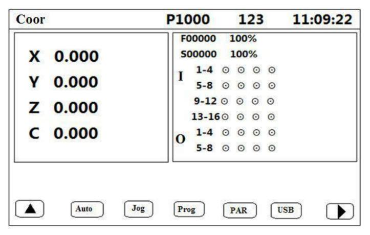
This is the interface showing after booting without boot picture. It shows the coordinates of each axis, F speed and rate, S speed and rate, as well as condition of input and output port. P1000 means the program currently running; 123 means the input method. You can get into the AUTO, JOG, PROG, PAR, USB as well as password interface from here.
