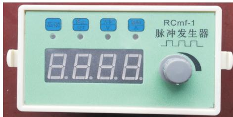
Cs10-3 controller can control stepper motor, servo motor, motor speed 0-4000rpm, square wave, stepless adjustable. Outside start stop, direction.it can realize external control, with speed regulation, round-trip, timing and length.
