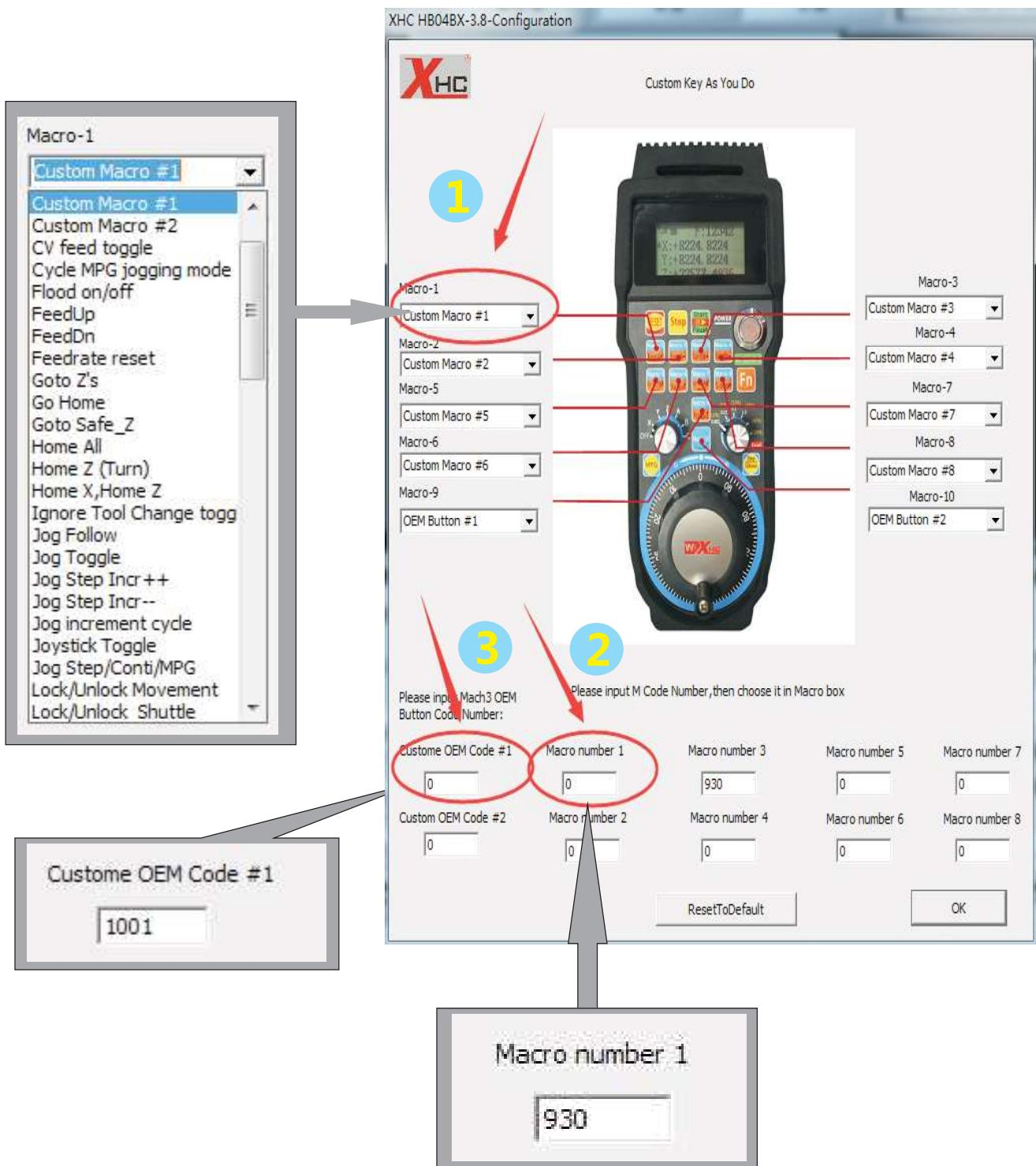
2. As shown in the figure below, you can select the extension function of the plug-in directly from the drop-down menu of macro-1, which will take effect after saving. If you write your own macro code file, you can set it according to the following illustrations:
