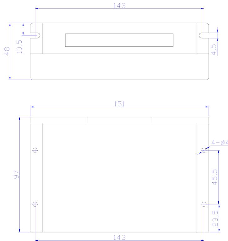
Figure 1: Mechanical specifications
